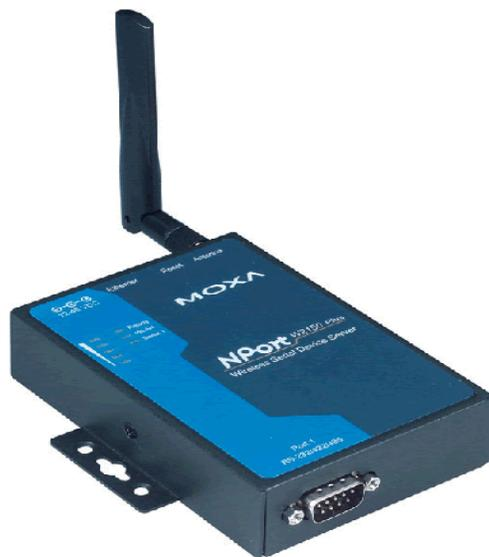
Step 1: Connect the Moxa unit to your computer's Ethernet port with the Ethernet cable
